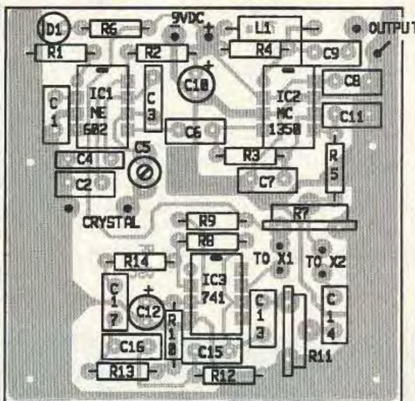
Figure 6. Parts placement.
