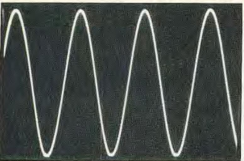
Photo C. Output waveform: AF from 741.
